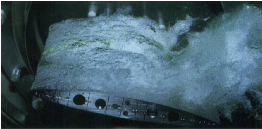
FIGURE 20. NACA 16 012; Re = 1\,000\,000 ; \sigma_v = 0.81 ; \alpha = 11^\circ , domain 4.
